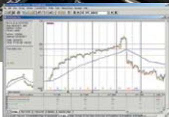
Zone Temperatures plotted with Heat Flow in a 10-zone oven
